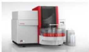
novAA Series Classical line source AAS with Dual Optics.
